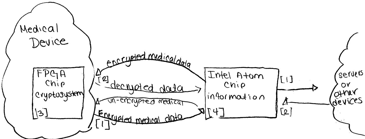
The Intel Atom chip communicates with the database or other devices to send the medical information from a medical device that has the FPGA chip within it, that is equipped with the crypto system.
