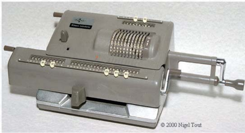
NCM/Busicom HL21 mechanical pinwheel calculator.
