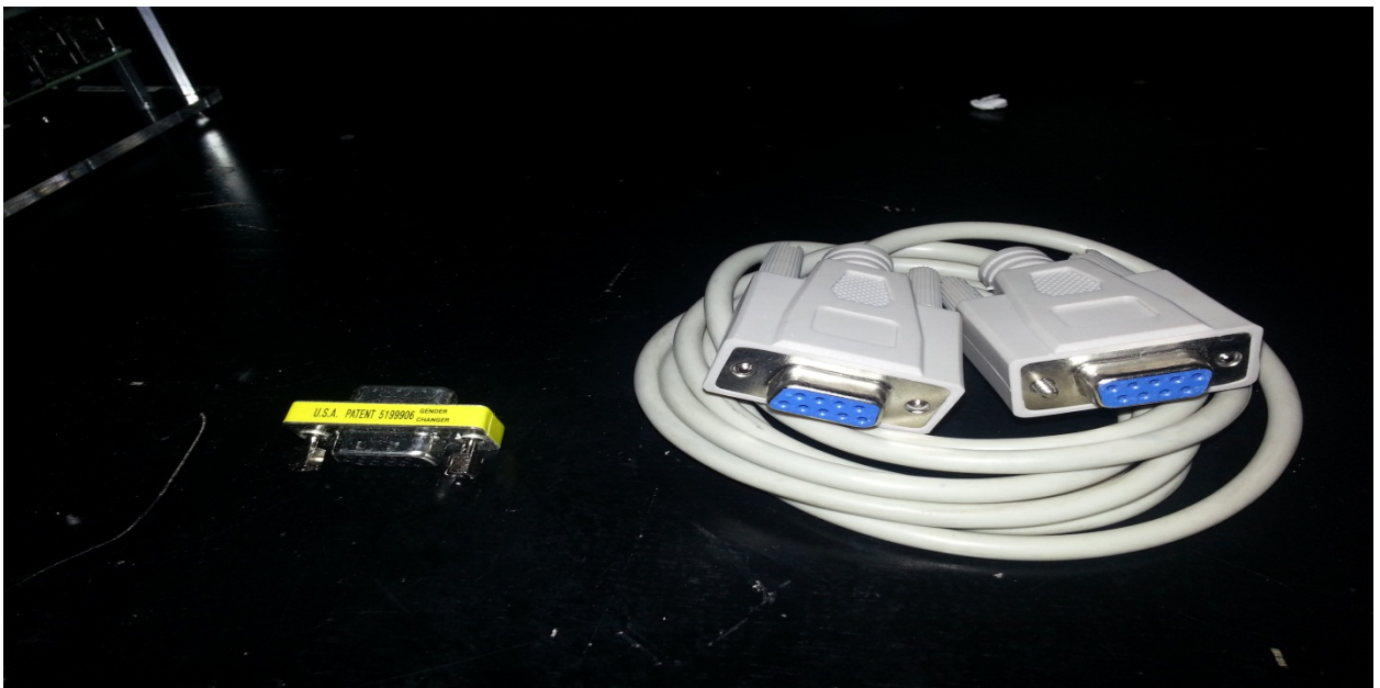
On right (female to female gender changer) Left (female to female serial cable)
