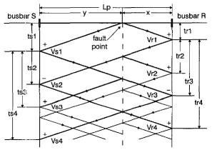
The distinction between the reflected wave from the fault point and that from the remote bus bar is vital.
