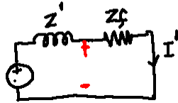
3-Phase Symmetrical Fault
