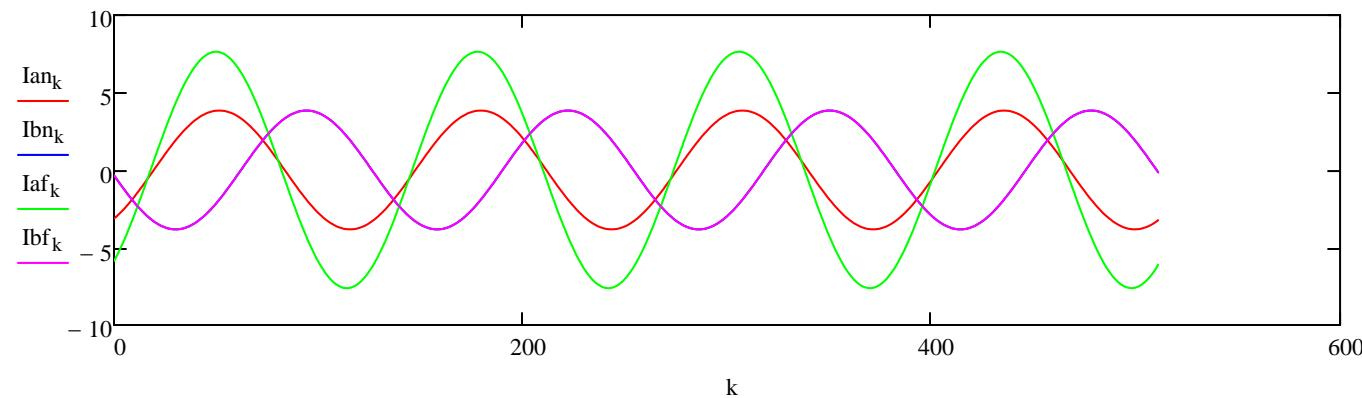
Let us make Normal (4 cycle)+ Fault (4 cycle) +Normal (4 cycle)
