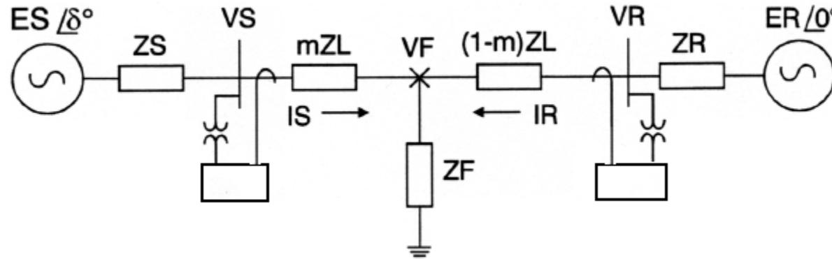
Fault Location  $d := 0.95$  $\delta := 0.001$  Voltage Phase Angle $es := 12000 \cdot e^{j \cdot \delta \cdot \text{deg}}$  Source S Voltage $er := 12000$  ~~er~~  $= 0$   $es = 1.2 \times 10^4 + 0.209i$  $Ssir := .3 \cdot e^{j \cdot -5 \cdot \text{deg}}$  Source S SIR(Soure Impedance Ratio)
