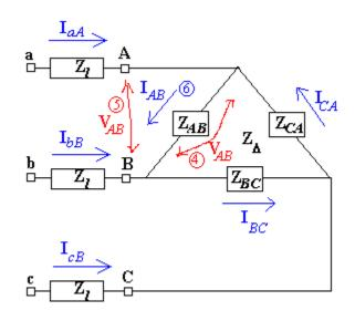
$V_{\phi}=V_{AB}, V_{BC}, \text{ and } V_{CA}$  (4)  $V_{l}=V_{AB}, V_{BC}, \text{ and } V_{CA}$  (5)  $I_{\phi}=I_{AB}, I_{BC}, \text{ and } i_{CA}$  $I_{l}=I_{aA}, I_{bB}, \text{ and } i_{cC}$
