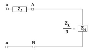
NOTE: The voltage across the impedance in this single-phase circuit is **not** the actual phase voltage across the impedance.  $V_{AB}$  is the actual voltage across a impedance. So we have to convert the voltage, after your calculation of  $V_{AN}$ , to  $V_{AB}$  for a delta-load phase voltage.
