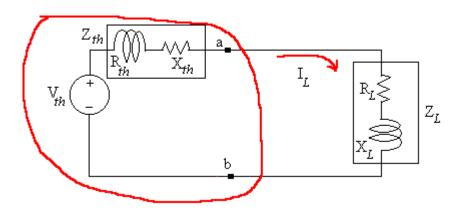
5. The only difference between two above circuits is that the sinusoidal circuit has complex elements. Let's assume the Thevenin voltage is with the phasor value of  $\overline{V}_{ih} = V \angle 0$ . Then, the
