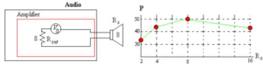
3. Now, we want to expand the maximum power transfer condition in the context of sinusoidal steady-state network. <u>Note</u> that the only power consumed is Real Power, so the term 'power' in the 'maximum power transfer' in the context of sinusoidal circuit, indicates *real power only*, as was in the constant source circuit.
