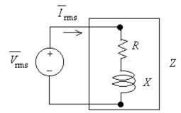
(1) From  $\overline{V}_{rms} = Z \cdot \overline{I}_{rms}$ ,  $\overline{S} = \overline{V}_{rms} \cdot \overline{I}^*_{rms} = \overline{Z}\overline{I}_{rms}\overline{I}^*_{rms} = \overline{Z}I_{rms}^2 = I_{rms}^2(R+jX) = R \cdot I_{rms}^2 + jX \cdot I_{rms}^2$ In this case:  $P = R \cdot I_{rms}^2$  and  $Q = X \cdot I_{rms}^2$ In other words, *P relates only to R, and Q, only to X*.
