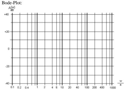
Do you see that the cut-off frequency (at –3dB) is  $\frac{1}{RC}$ ? or  $w_c RC = 1.0$
