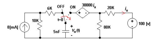
4. The switch in the circuit has been in position a for a long time. At t = 0, the switch moves instantaneously to position b. Find  $v_0(t)$  for  $t \ge 0$ .
