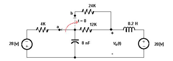
5. The switch in the circuit has been in the closed position for a long time, and at t=0, it is opened instantaneously. Find i(t) for t>0. (A final exam problem of Spring 2004)
