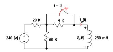
3. The switch in the circuit has been in the OFF position for a long time. At t = 0, the switch moves instantaneously to the ON position. Find  $v_0(t)$  for  $t \ge 0$ .
