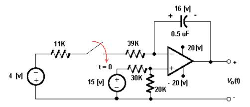
2. The switch in the circuit has been closed for a long time. The switch opens at t=0. Find the numerical expressions for  $i_0(t)$  and  $v_0(t)$  for  $t \ge 0$ .
