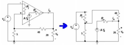
(b) Let's apply the node-voltage method to the right circuit.
