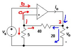
(b) Constraints and hidden values: by the ideal op amp model,  $V_1=V_s$  and  $V_0=V_2$ .
