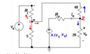
(c) @ node 1:  $\frac{V_1 - V_s}{R_i} + \frac{V_1}{5} + \frac{V_1 - V_o}{40} = 0$  (Since  $V_o = V_2$ ). with  $V_s = 1$ --->  $\frac{V_1 - 1}{2 \times 10^6} + \frac{V_1}{5} + \frac{V_1 - V_o}{40} = 0 \implies (V_1 - 1) + 0.4 \times 10^5 V_1 + 0.05 \times 10^6 (V_1 - V_0) = 0$
