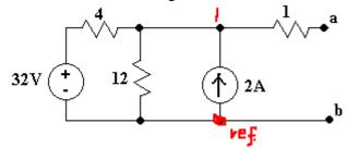
Therefore, @node 1:  $\frac{V_1 - 32}{4} + \frac{V_1}{12} - 2 = 0 - --> V_1 = 30 V - ---> V_{th} = 30 V$
