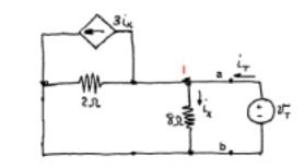
Constraint:  $i_x = \frac{V_1}{8}$ ,  $V_1 = V_T$ .
