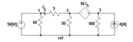
2. Since we already know V<sub>1</sub>=50 V by the source. We do not need equation at node 1. 3. At the node 2, we can easily express the current to the left [i.e.,  $\frac{V_2 - 50}{5}$ ] and the current down to the reference [i.e.,  $\frac{V_2}{50}$ ] easily. But how do we express the current to the right?
