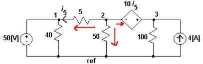
4. Remember that node-voltage method is KCL in disguise? Here the "one more step" enters in. Do you see that the current to the right (at node 2) is the sum of the two current at the next node (i.e., node 3)?
