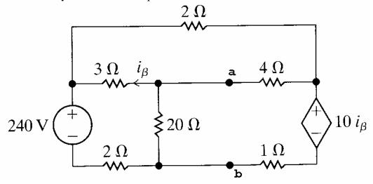
2. Use PSpice to find the Thevenin equivalent circuit at the terminals **a** and **b** for the network above. Be sure to provide all the circuit diagrams and simulation results, and the final Thevenin equivalent circuit diagram, in your report.
