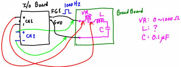
4. Parallel RLC case as in FIG.4 using Mobile Studio Lab. Do the same processes (a) and (b) (but with [1/2RC]<sup>2</sup> vs. [1/LC]) as in the RLC series case.
