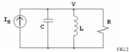
The node voltage equation for the above circuit is:
