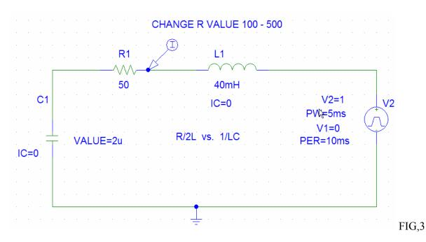
Check if you can make three damping conditions by changing the value of R between 100 and 500 ohm. Remember that  $[R/2L]^2$  vs. [1/LC] determines the damping condition. Bigger  $[R/2L]^2$  means more damping, overdamping condition.
