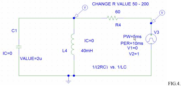
Check if you can make three damping conditions by changing the value of R between 50 and 200 ohm. Remember that  $[1/2RC]^2$  vs. [1/LC] determines the damping condition. Bigger  $[1/2RC]^2$  means more damping, overdamping condition.
