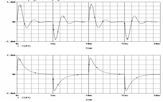
2. Simulation of Parallel RLC as in FIG.2 can be changed in the following schematic by applying source transformation. We can do it without change in PSpice, but since we are doing the same thing using Mobile Studio which does not have current source, it would be better work with voltage source circuit with series resistance instead of current source with parallel resistance.
