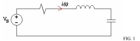
The loop KVL equation for the current of the above circuit is:
