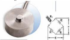
A load cell is typically an electronic device that is used to convert a force, sensed the deformation resulted from the exerted force in a strain gauge, into an electrical signal. A load cell consists of four strain gauges in a bridge configuration, but is also available with one or two strain gauges.
