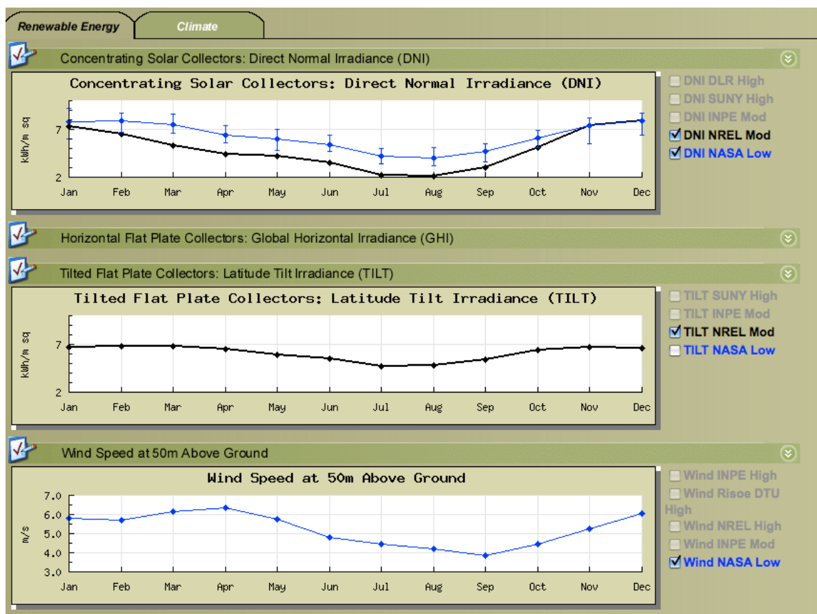
Figure 12. This figure shows the time series data accessed through RREX by using the Graph Data option on the main window. This image illustrates how users can display data from multiple sources by checking the boxes next to more than one data layer (DNI graph), how graphs can be hidden by clicking on the label bar (GHI), and how unavailable data layers are grayed out.
