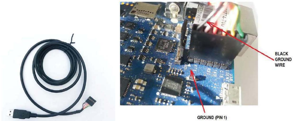
The next step tests the cable with Galileo Gen 2 board. By the way, to run a Linux console with the cable, we need to install the software on a computer in order to open a serial channel with Galileo Gen 2. The software we need depends on our operational system and our preference. This step explores **putty** for Windows, **minicom** for Linux, and **screen** for Mac OS. Note that **screen** is also available on Linux, and **minicom** is also available in Mac OS.
