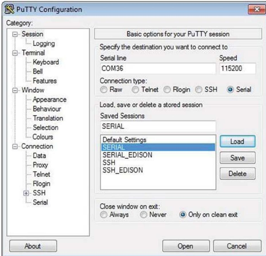
**Figure 1-21.** Configuring putty to open the Linux console
