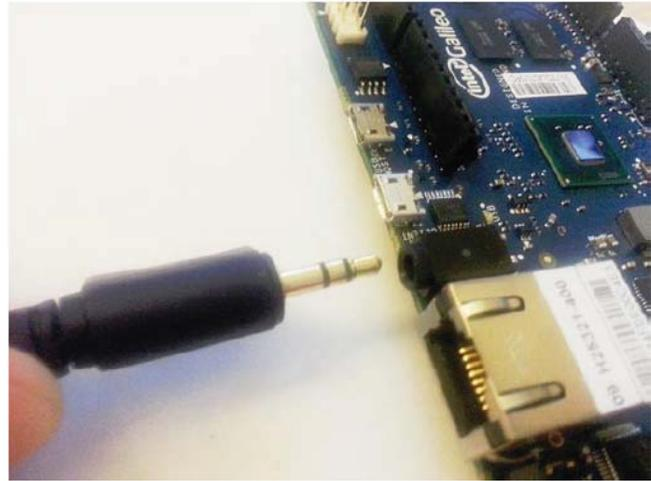
The next step tests the cable with Galileo Gen 1 board. By the way, to run a Linux console with the cable, we need to install the software on a computer in order to open a serial channel with Galileo Gen 1. The software we need depends on our operational system and our preference. This step explores **putty** for Windows, **minicom** for Linux, and **screen** for Mac OS. Note that **screen** is also available on Linux, and **minicom** is also available in Mac OS.
