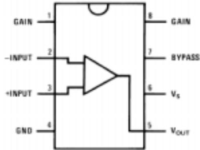
2. Draw a connection diagram for a Gain 200 audio amplifier. Attach a speaker at the output.
