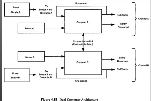
• When a failure is detected, the computer software generates a disconnect output that must reconfigure the system to a fail-safe condition.
