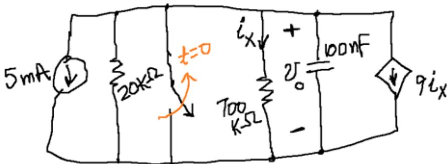
Before  $t < 0$ , all current flows through the shorted line, voltage is zero. So the initial voltage in the capacitor is zero.
