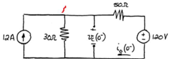
$v_1 = v_0$  and  $i_0$  = current through 50 ohm resistor
