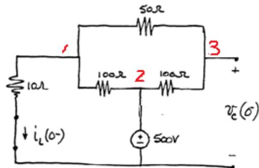
$$V_2 = 500 \text{ and } V_3 = v_0, i_0 = V_1/10$$
