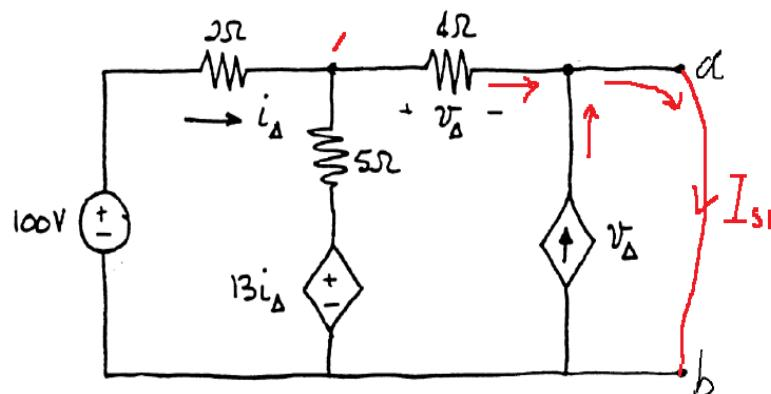
$$I_{sc} = v_{\Delta} + V_1/4 \quad \text{but } v_{\Delta} = V_1$$
