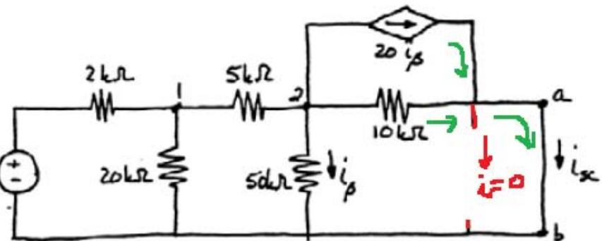
$$i_{SC} = V_2/10 + 20*i\beta = V_2/10 + 20*(V_2/50) \quad [\text{mA}]$$
