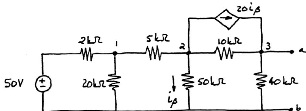
$$V_{th} = V_3$$
