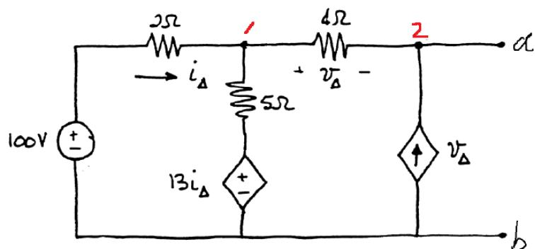
$$V_{th} = V_2$$
