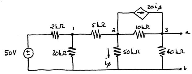
2. (Problem 4.66) Find the Thevenin equivalent with respect to the terminals a and b for the circuit below.
