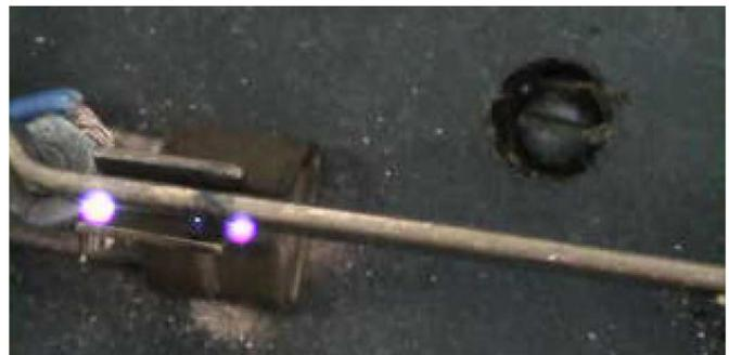
Fig. 2. Arc/spark generation in the blade contact of a knife switch by rubbing actions.
