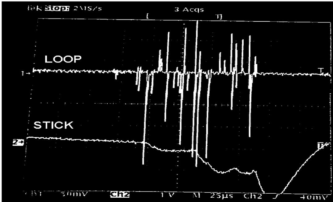
Fig. 8. Signal captured by the loop and the stick antennas with  $25 \mu\text{s}/\text{div}$ .
