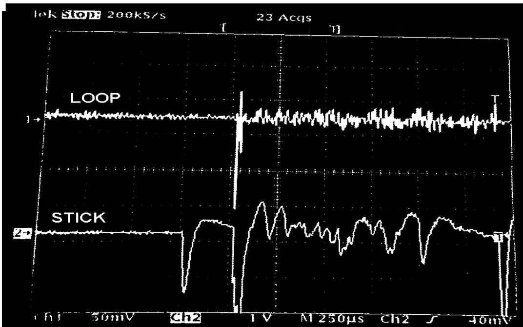
Fig. 10. Inception of radiation signals captured by two antennas with 0.25 ms/div.
