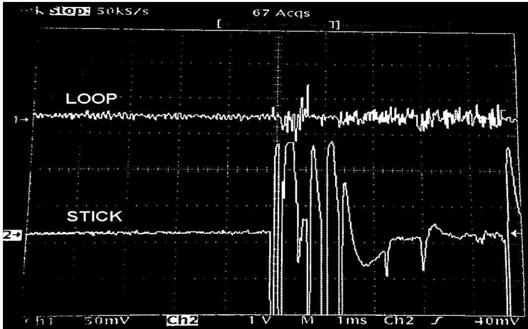
Fig. 9. Inception of radiations captured by two antennas with 1 ms/div.
