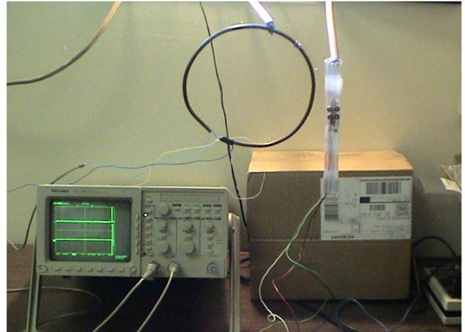
Fig. 1. Loop antenna and a stick antenna were used in radiation capture experiments.
