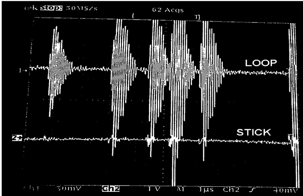
Fig. 7. Signal captured by the loop and the stick antennas with  $1 \mu\text{s}/\text{div}$ .
