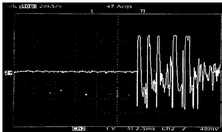
Fig. 4. Second arc/spark signal of Fig. 3, but in a shorter time/div for a detailed waveshape.
