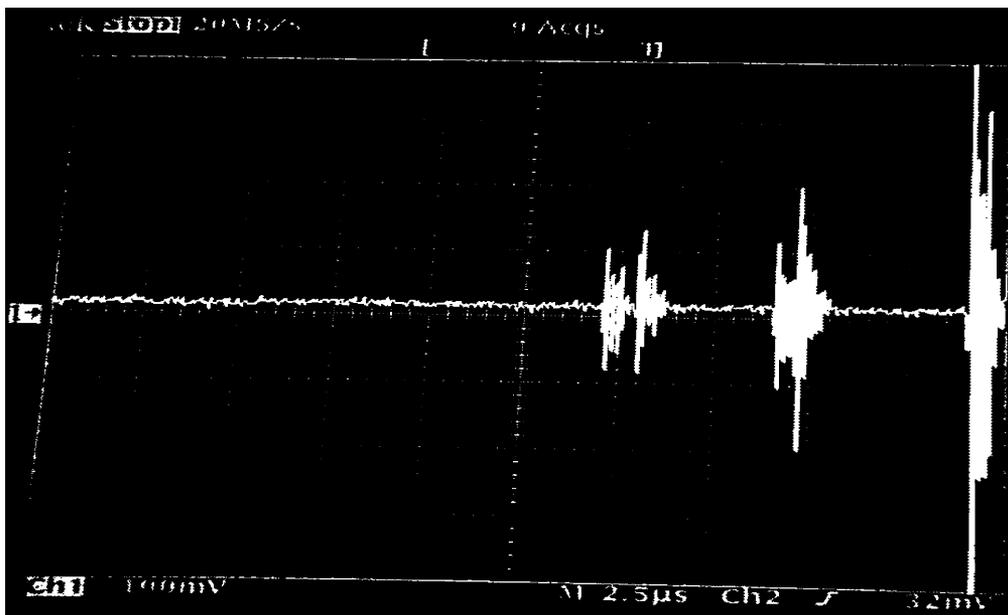
Fig. 6. Loop antenna-captured signal of radiated bursts, some with even less than a 1- $\mu$ s pause period.
