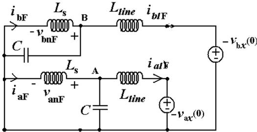
Fig. 7. Simplified circuit diagram of ABE fault.
