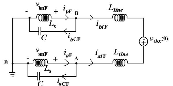
Fig. 5. Further simplified circuit for AB fault.
