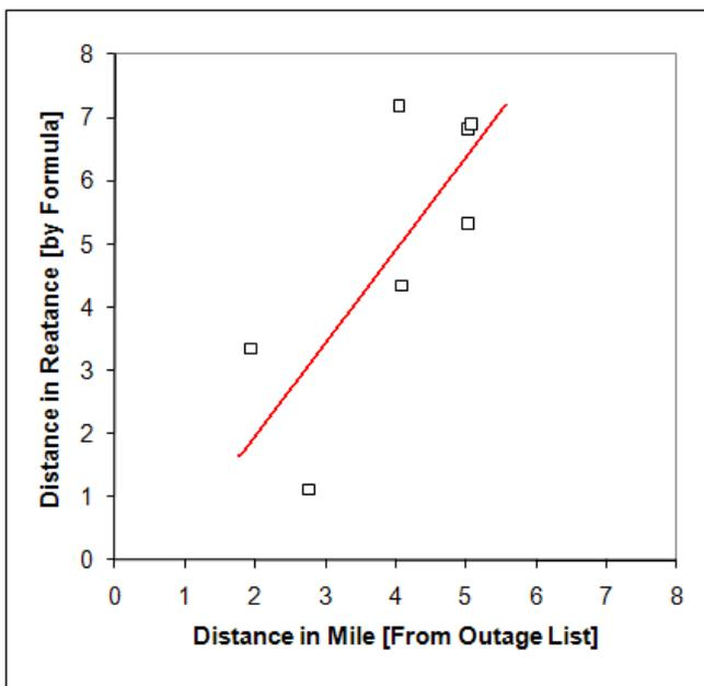
Fig. 11. Calculated fault distance vs. true fault distance
