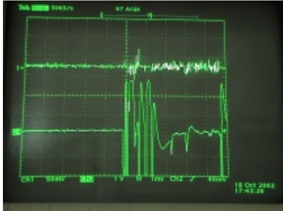
Figure 6: Actual photoshots of the captured signals by the stick and loop antennas. Top tracings are from loop antenna and, the bottom ones, from stick antenna.
