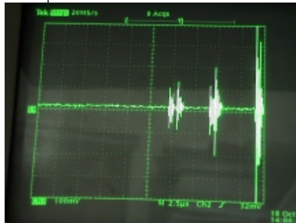
Figure 5: Actual photoshot of teh captured signal from the loop antenna.
