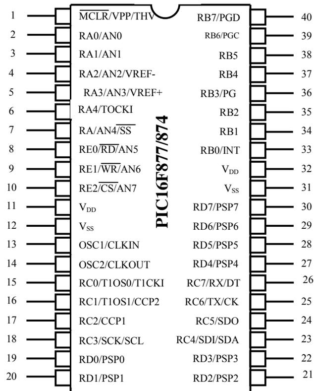
Fig 1. PIC 16F877 IC Package: DIP
