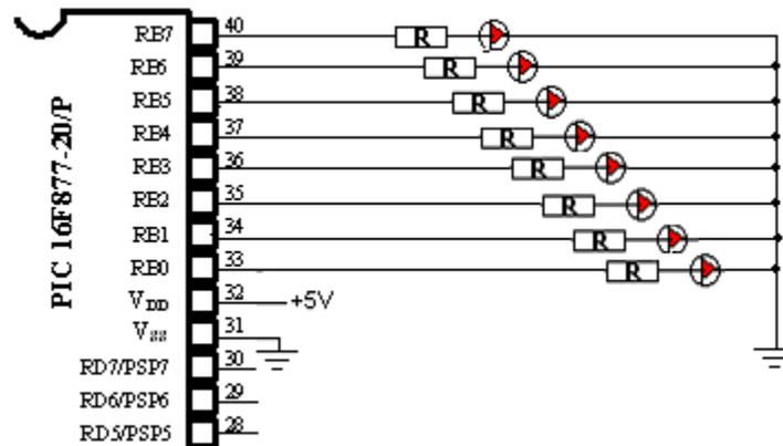
Fig 7. Example of LEDs on PORTB
