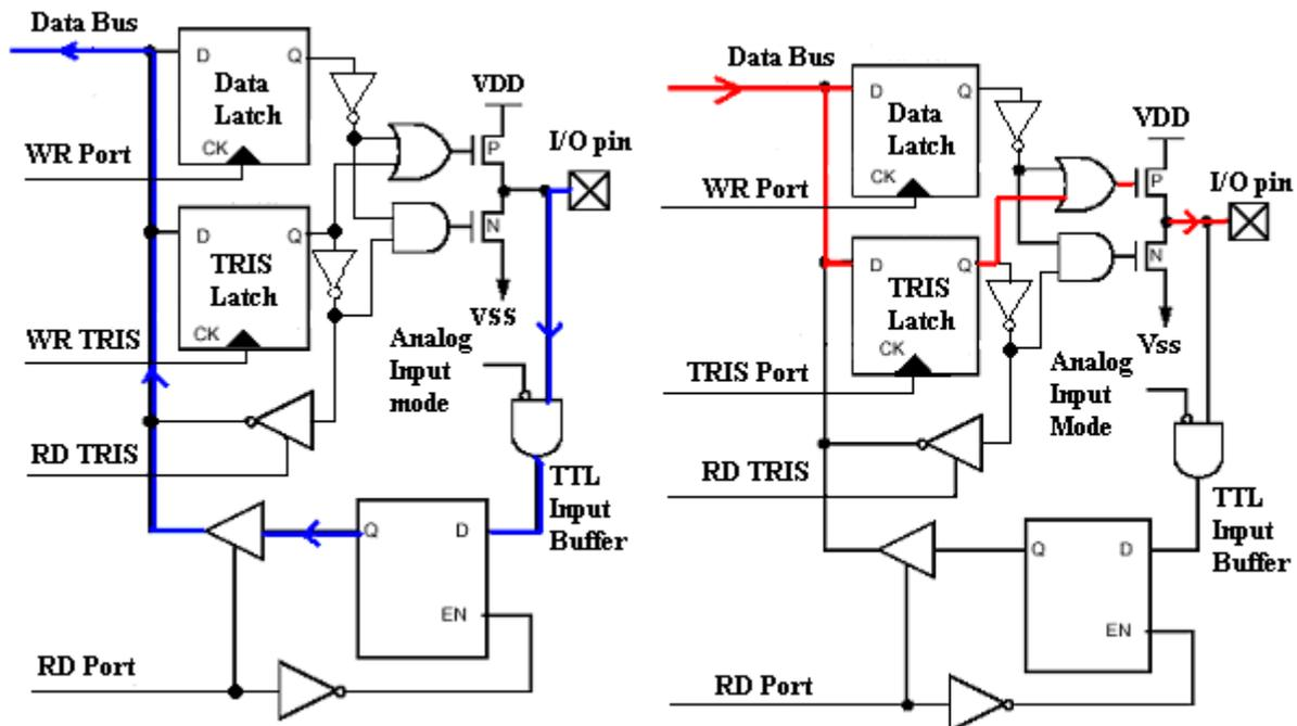
Fig 6. Input (left) and Output (right) operation of a port register.
