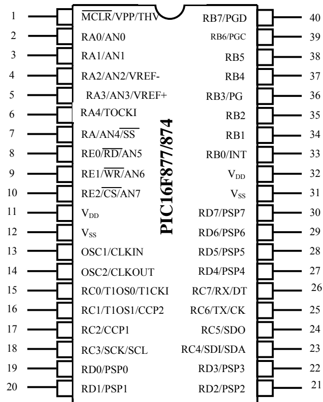
Fig 1. PIC 16F877 IC Package: DIP
