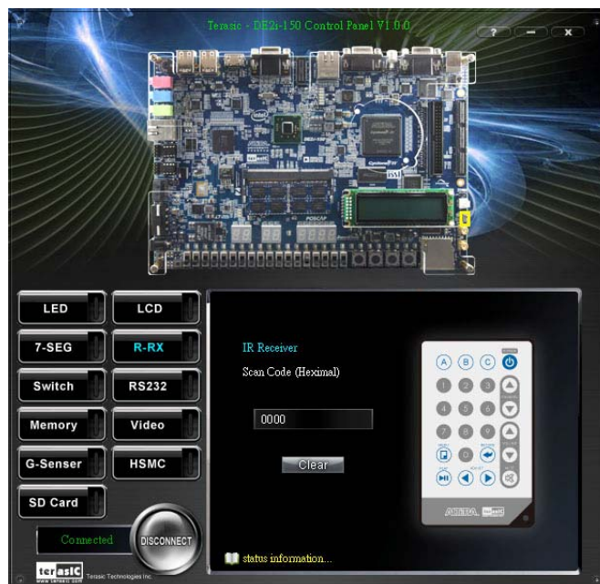
Figure 2-12 Testing the IR receiver using remote controller
