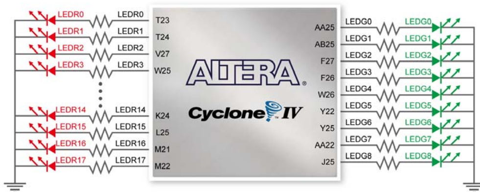
Figure 3-10 Connections between the LEDs and Cyclone IV GX FPGA
