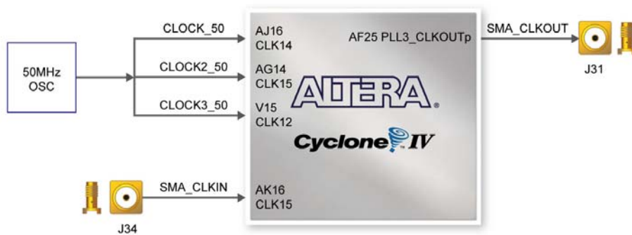
Figure 3-12 Block diagram of the clock distribution
