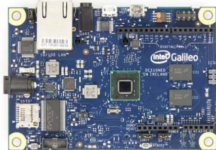
**Arduino-Compatible Development Board featuring Intel Architecture**
