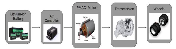
In this conceptual design, the Lithium Ion battery supplies DC power using electrochemical processes. This DC is first converted into AC by the controller, since the Permanent Magnet operates in AC. The controller also regulates the amount of current delivered to the PMAC motor (battery management). It avoids too much power pull when the batteries are hot, cold, or close to empty). This allows the PMAC to operate at a very high efficiency.
