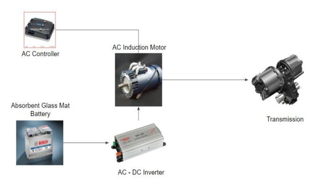
**The Motor**: The motor in this design is an AC induction motor. This is the type of motor used in one of the most popular EVs on the market, the Tesla Model S. It uses an inverter to convert the DC power of the battery to AC power. It is highly efficient over wide ranges of rpms and loads, moderately priced and aids with regenerative braking.
