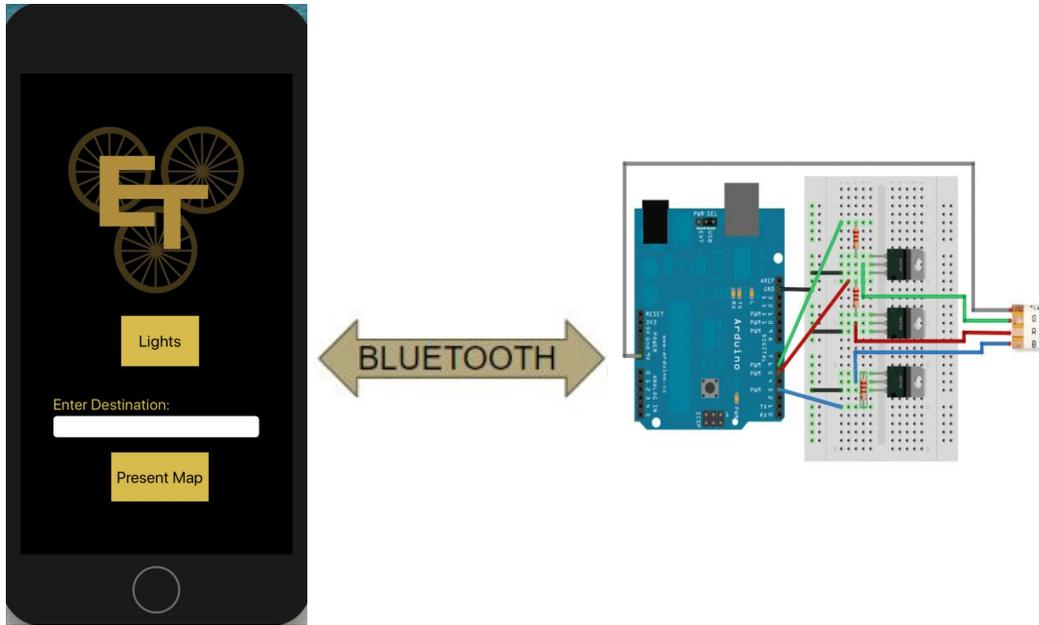
Each “buttonTapped” function above correlated to a different light which was signified by a different hexadecimal input. Orange was 0x31, red was 0x32, white was 0x33, and off was 0x30 in the swift code. In the Bluetooth code for arduino, these inputs equated to 1, 2, 3 and 0 respectively as shown below.
