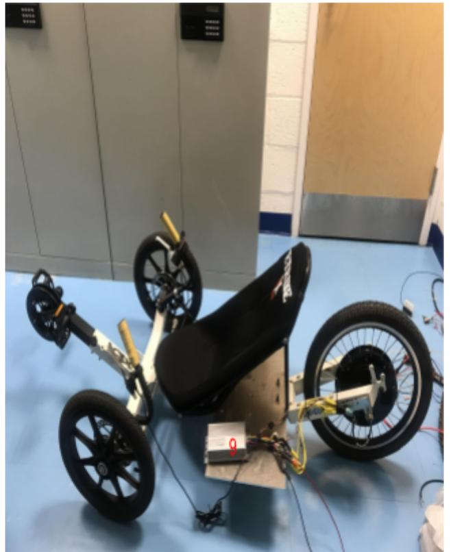
1. KMX Hardshell Bucket Seat with an easy angle and frame position adjustment.
