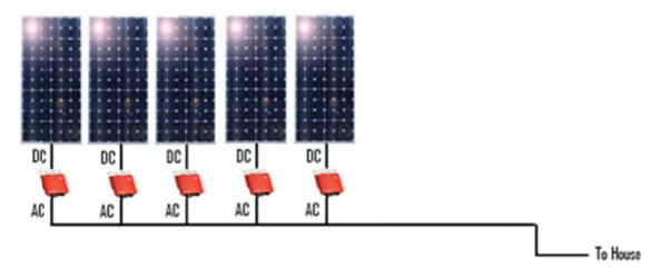
Figure 1 micro inverter conceptual design
