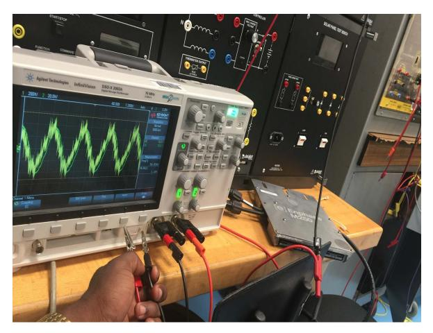
Figure 5 Testing for the output AC signal from two micro inverter connected in parallel
