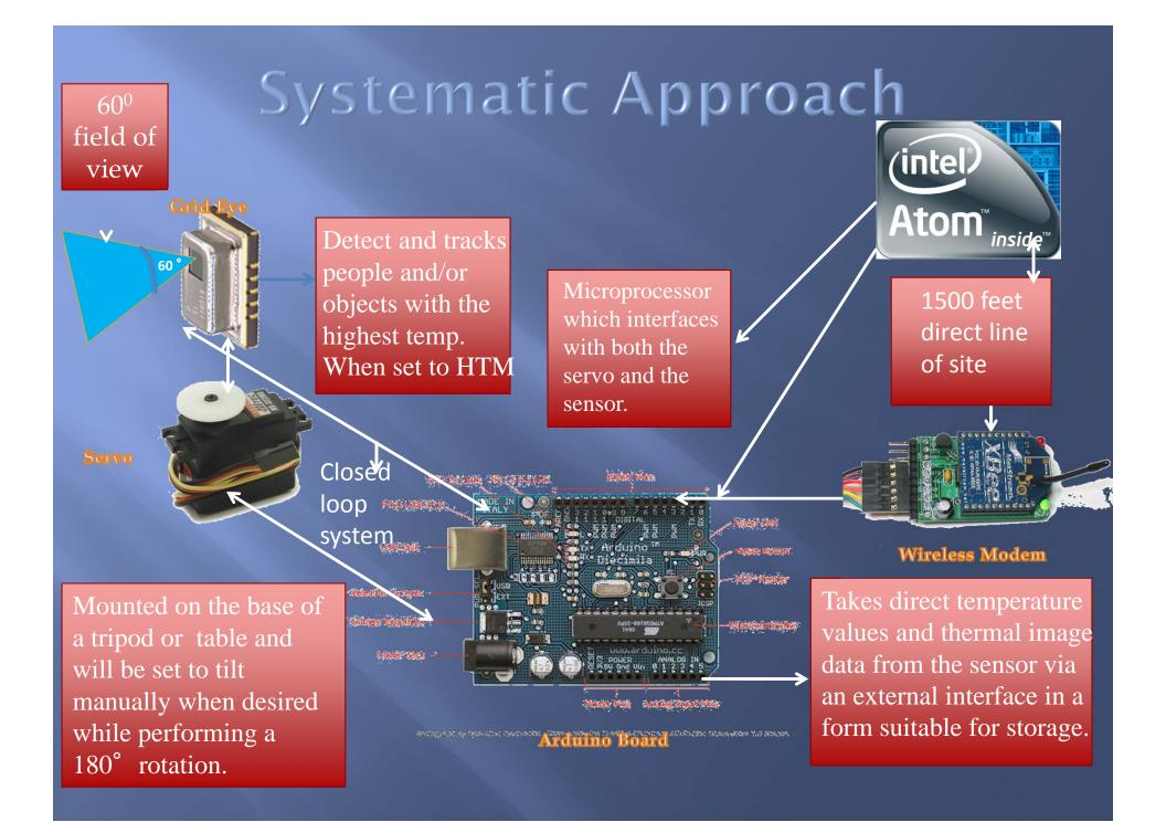
We expect to have a working prototype of the device by the date of EECE day April 2013. The device is expected to detect an object, produce a thermal image and display that image on a computer monitor. When more than one objects with different temperature are present, the sensor will track the object with the highest temperature once set on the HTM by the end user on the base computer.
