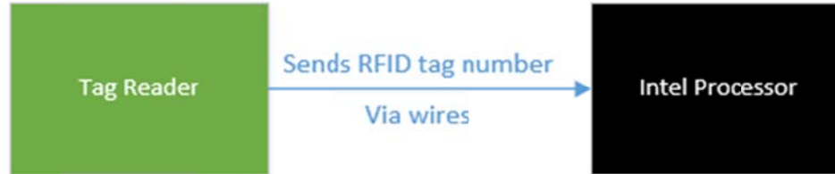
Figure 2: RFID Reader Tells Processor Which Tags It Senses
