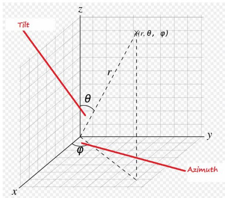
*Fig.1 Spherical coordinate system showing azimuth and tilt*
