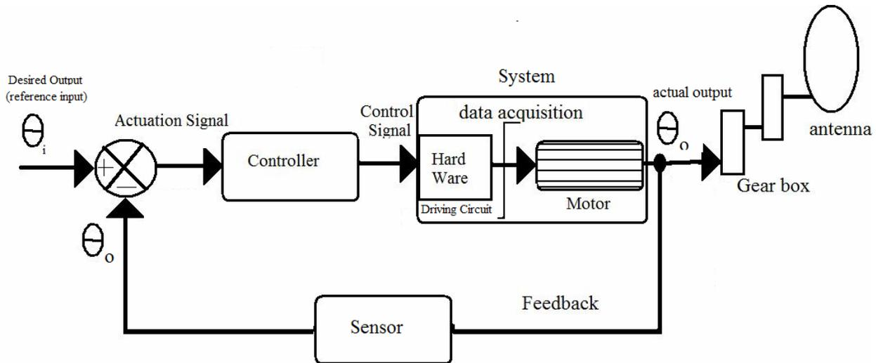
*Fig.4 Closed Feedback Loop for motor position control*
