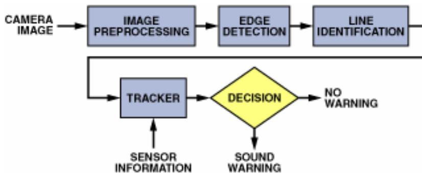
Figure 3b: LDWS Camera solution schematic
