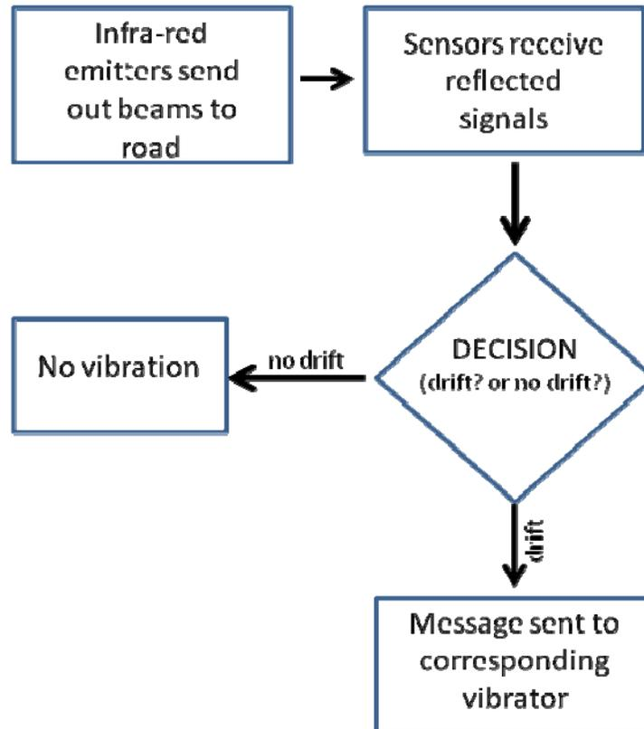
Figure 3a: LDWS Infra-red technology schematic
