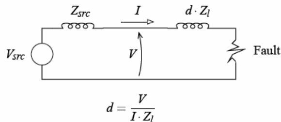
Where  $d$  is the distance to the fault,  $Z$  is the impedance value,  $I$  is the current and  $V$  is the voltage. The Arc Voltage Estimation consists of the fault location, the estimated fault type, and estimating the arc power and energy.
