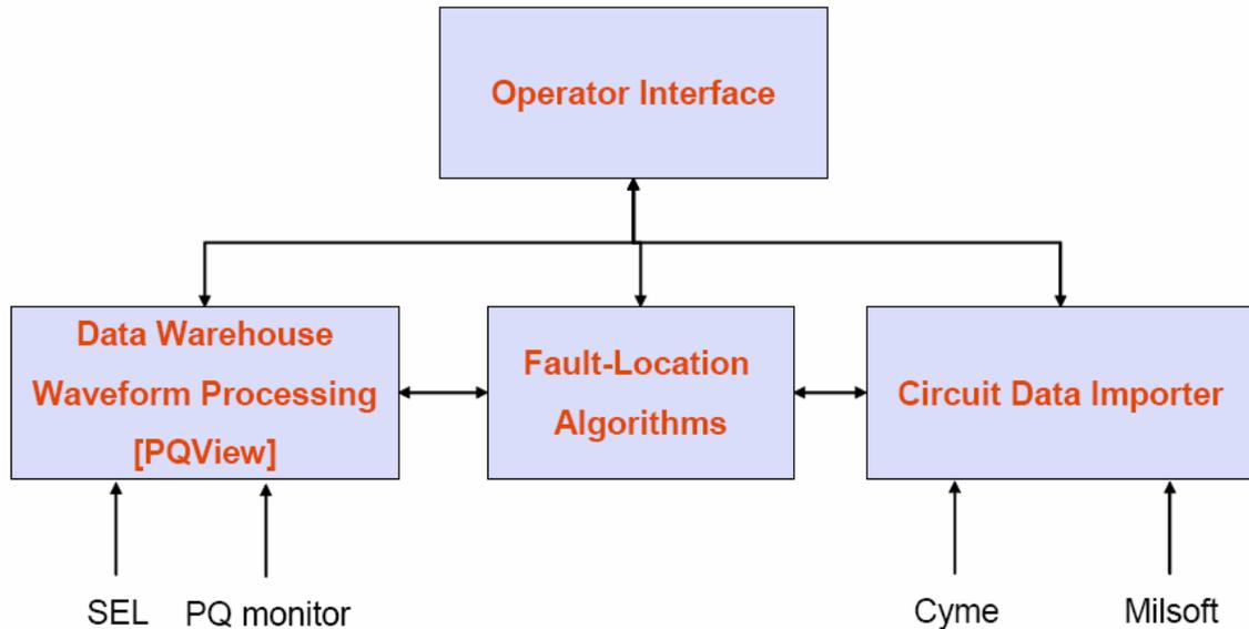
**EPRI diagram of an integrated fault location system**
