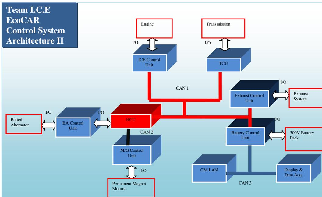
Fig.4 Architecture II of real time communication using CANs
