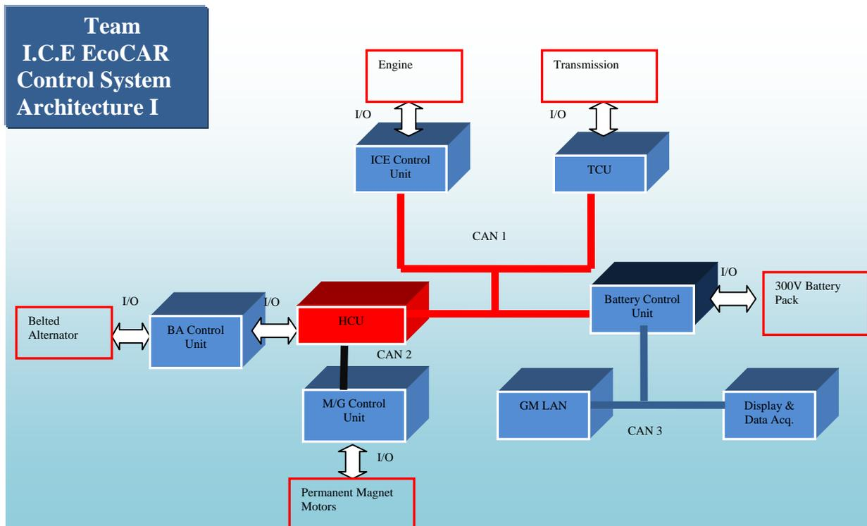
Fig.2 Architecture I of real time communication using CANs
