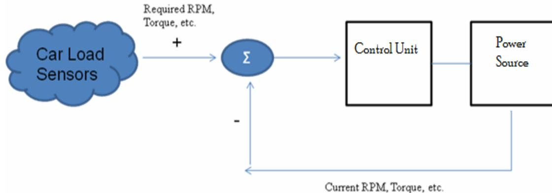
Fig. 3 Feedback loop for Hybrid Control Unit
