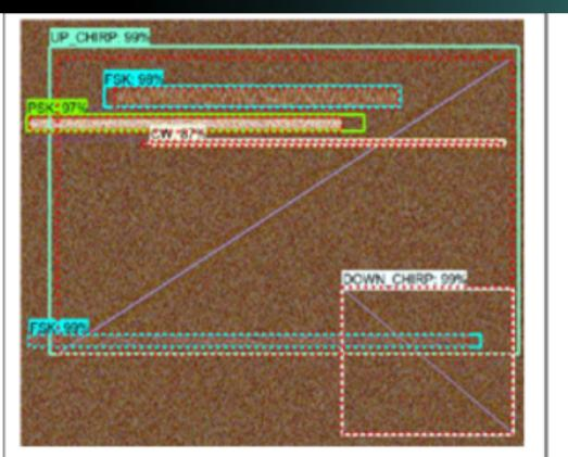
Figure 2 - Image based CNN signal detection and classification
