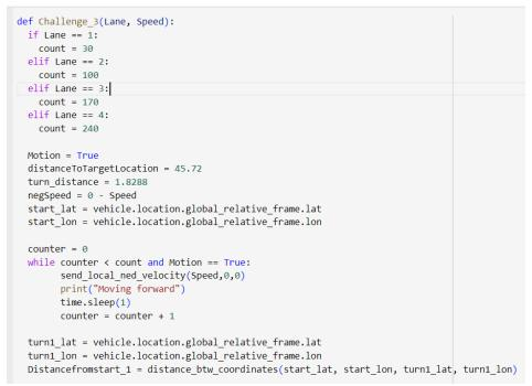
We calculate how much distance the UGV covered in the first part of the challenge using the "distance\_btw\_coordinates" function and store it in the variable "Distancefromstart\_1". We then send commands to turn the UGV right, move forward for 2 yards then turn left.
