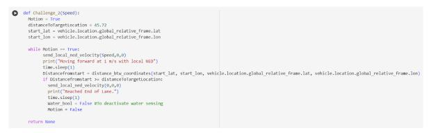
Before the loop begins we store the coordinates of the UGV at the start of the challenge. In each iteration of the loop we use the function "distance\_btw\_coordinates()" to calculate the distance between the starting coordinates and the current coordinates.
