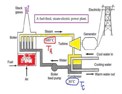
Heat Rate, Heating Value, Fuel Rate
