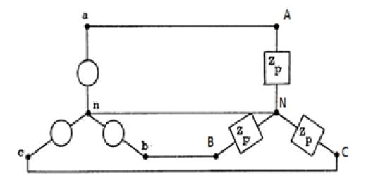
A 440-V rms (line voltage) three-phase three-wire system feeds two balanced Y-connected loads. One load is an induction motor which may be represented by an impedance of  $10 + j5\Omega$  per phase. The other is a lighting load equivalent to  $15\Omega$  per phase. Find the average power: (a) delivered to the lighting load; (b) delivered to the induction motor
