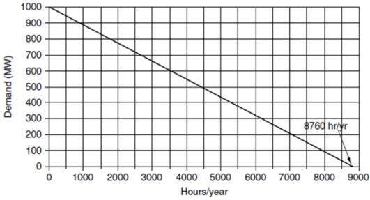
To serve the customers, the company runs 3 power plants: 500 MW coal-steam to cover the base load, 300 MW combined-cycle for the intermediate load, and 200 MW gas turbine for the peak load. The cost parameters of the power plants are as shown below. The fixed charge rate (FCR) for the capital cost is 0.16 per year.
