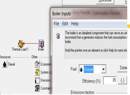
$$c_{\text{boiler,mar}} = \frac{3.6c_{\text{fuel,eff}}}{\eta_{\text{boiler}} \text{LHV}_{\text{fuel}}}$$
