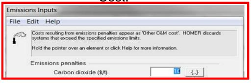
To cap carbon dioxide emissions, click the CO2 checkbox in the lower half of the Emissions window and enter the maximum allowable emissions in kg/yr. To apply a carbon tax enter the penalty in \$/tonne in the top half of the window. Just be sure to enter it in terms of \$/tonne of CO2, not per tonne of carbon.
