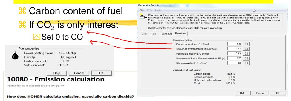
If the system you are modeling consumes fuel, HOMER calculates the total annual carbon input by multiplying the fuel consumption by the carbon content of the fuel. It assumes that all that carbon gets emitted as either unburned hydrocarbons, CO, or CO2. You enter the emissions factors for unburned hydrocarbons and CO, so HOMER can calculate how much of the total carbon gets emitted in those two forms. The rest gets emitted as CO2.
