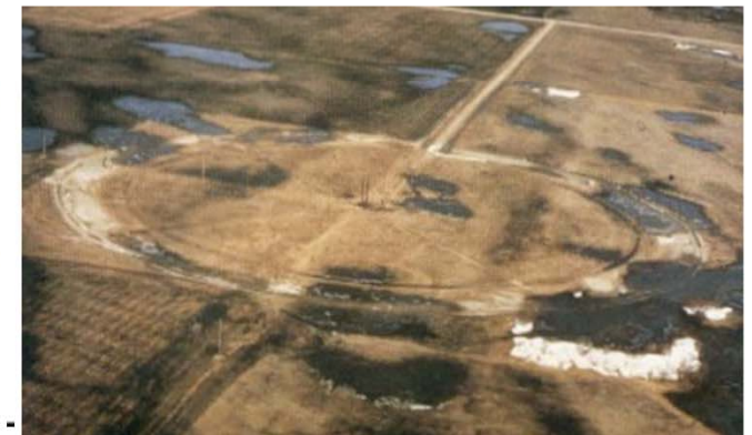
Ring of ground electrodes, 300 m radius, for 500 kV HVDC (Manitoba).
